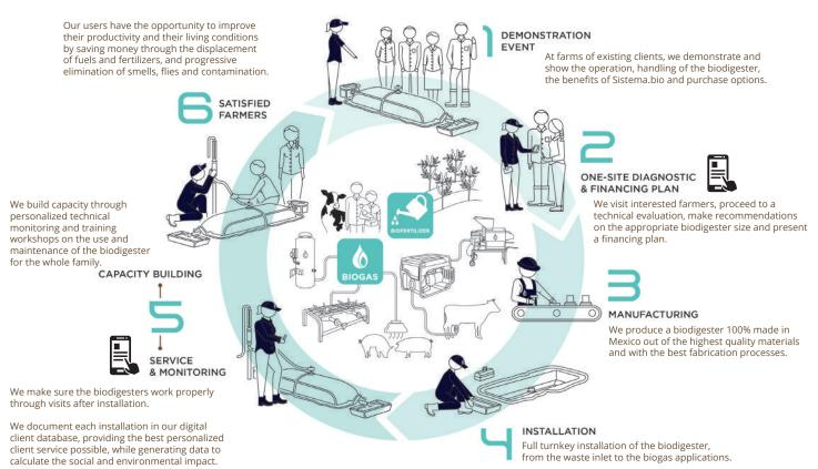
The Sistema.bio program is based on our easy-to-install technology, combined with financing packages, training and monitoring. It provides a turnkey package which produces biogas and organic fertilizer (biol) at the local, regional or national level. This Sistema.bio technology generates important benefits in the fight against climate change, health, savings, and productivity. These benefits are in turn aligned with national and international sustainability goals.
