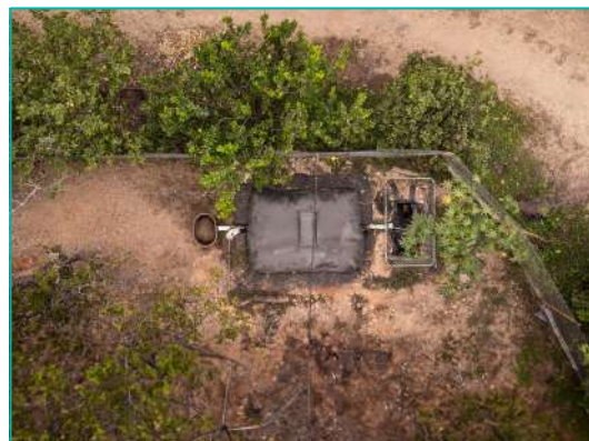
Sistema 8 Area Required: 8.5 x 4.0 m Biogas: 2.4 m 3 /day*
