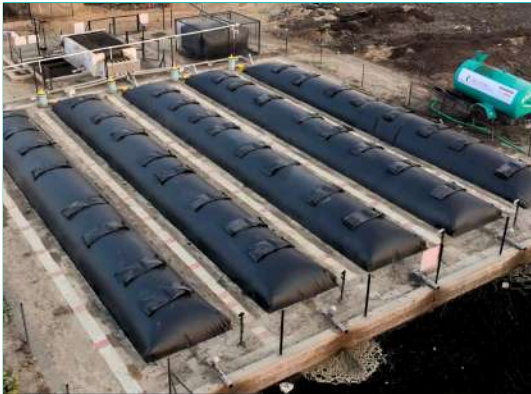
Sistema 200 Area Required: Sis 40 X 5 Biogas: 65 m3/day*
