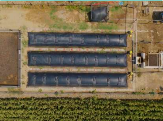
Sistema 120 Area Required: Sis 40 X 3 Biogas: 39m3/day*
