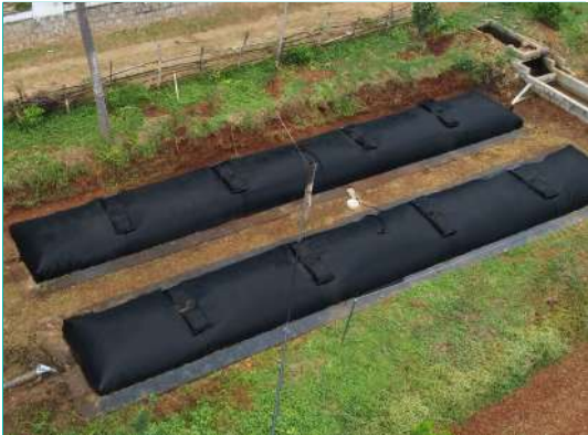
Sistema 80 Area Required: Sis 40 x 2 Biogas: 26 m3/day*
