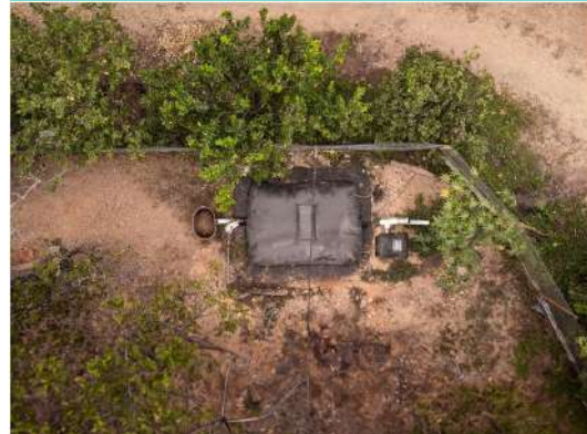
Sistema 8 Area Required: 3.4 X 6.2 m Biogas: 2.4 m 3 /day*
