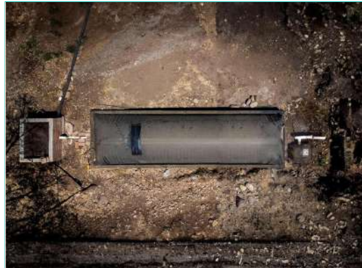
Sistema 20 Area Required: 3.4 X 12.2 m Biogas: 6.7 m 3 /day*
